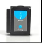
The internal humidity sensor utilizes a dielectric polymer to absorb water molecules. As more water molecules enter, the capacitance changes proportionally to the relative humidity value. Using this technique an accurate relative humidity value is calculated.
