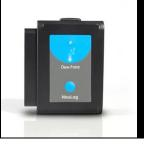
Your dew point sensor needs to be connected to a WIFI-201 module. The WIFI-201 module will create a closed NeuLog wifi network which will stream the NeuLog data to a device of your choosing. Once your device is wirelessly connected to the NeuLog network you can run experiments and collect data through a browser of your choosing.
