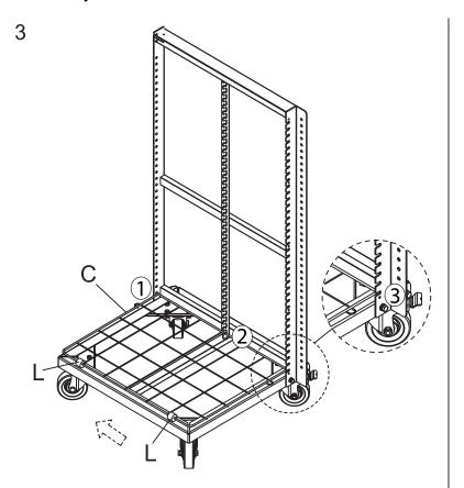
① Insert back, left corner of shelf into bottom hole on the back panel, align with corresponding center notch 2 and slot on right side of back panel. ③
