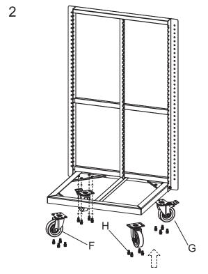
Attach Casters (F & G) to bottom of Base (B) using Bolts (H).
