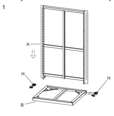
Attach Back Panel (A) to Base (B) using Bolts (H).
