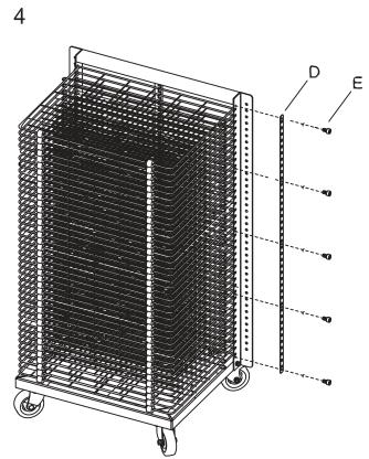
Secure shelves by attaching Side Bar (D) and tightening Socket Head Cap Screws (E) with Allen Wrench.
